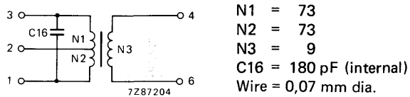
Fig. 11 I.F. bandpass filter (L1). TOKO sample no. 7 MC-7 P.
